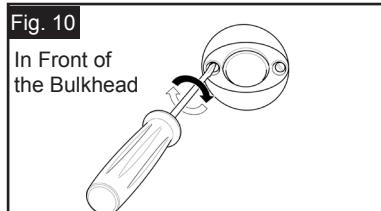
**STEP 4.** Place the housing through the hole (Fig. 9). Install by tightening the 2 screws in the front face until the flange is securely mounted to the bulkhead (See Fig. 10) i.e. touching at all points around the circumference. Ensure that the screw holes are on a horizontal plane.
