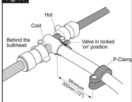
**Note** In order to securely fasten the unit, ensure that the p clamp mounting surface is at least 19mm (3/4") minimum thickness.
